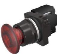
30mm BlackMax, Epoxy Coated Corrosion Resistant Complete Metal Unit Illuminated Push-Pull Operator Transformer type, 240V AC LED Lamp Mushroom Head Cap Small 1 3/4" (44.5 mm) Plastic, Red 3 Position Momentary UL Listed, CSA Certified NEMA 1,3,3R,4,4X,12,13 & Automotive Standards
