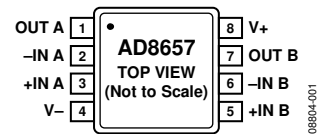
Figure 1. AD8657 Pin Configuration, 8-Lead MSOP
