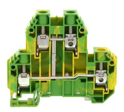
Protective-earth double-level terminal, Screw connection, Mounting type: Mounting rail TS 35/7.5, Rated cross-section: 10 mm², Width: 10.1 mm, Colour: Green-yellow
