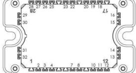
Pins 29/30/31/32 must be shorted together Pins 26/27/28/22/23/25 must be shorted together to achieve a phase leg Pins 16/18/19/20 must be shorted together
