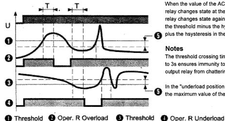
When the value of the AC / DC voltage reaches the set threshold value the output relay changes state at the end of the time delay T1 (contacts 11 & 14 open). The relay changes state again (contacts 11 & 14 closed) when the voltage falls below the threshold minus the hysteresis in the overload position, or above the threshold plus the hsysteresis in the underload position.
