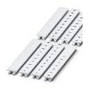
Zack marker strip, Strip, white, labeled, can be labeled with: CMS-P1-PLOTTER, printed horizontally: consecutive numbers 1 ... 10, 11 ... 20, etc. up to 91 ... 100, mounting type: snapped, for terminal block width: 8.2 mm, lettering field size: 10. 5 x 8.15 mm, Number of individual labels: 10
