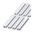
Marker for terminal blocks, Strip, white, labeled, can be labeled with: CMS-P1-PLOTTER, horizontal: L1, L2, L3, N, PE, L1, L2, L3, N, PE, mounting type: snapped, for terminal block width: 8.2 mm, lettering field size: 10.5 x 8.15 mm, Number of individual labels: 10
