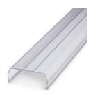
Cover profile, for covering terminal strips, snapped onto APT-ME cover profile carrier or APH-ME end bracket. A cover profile carrier should be positioned at the ends and at intervals of around 40 cm. Length supplied: 1 m
