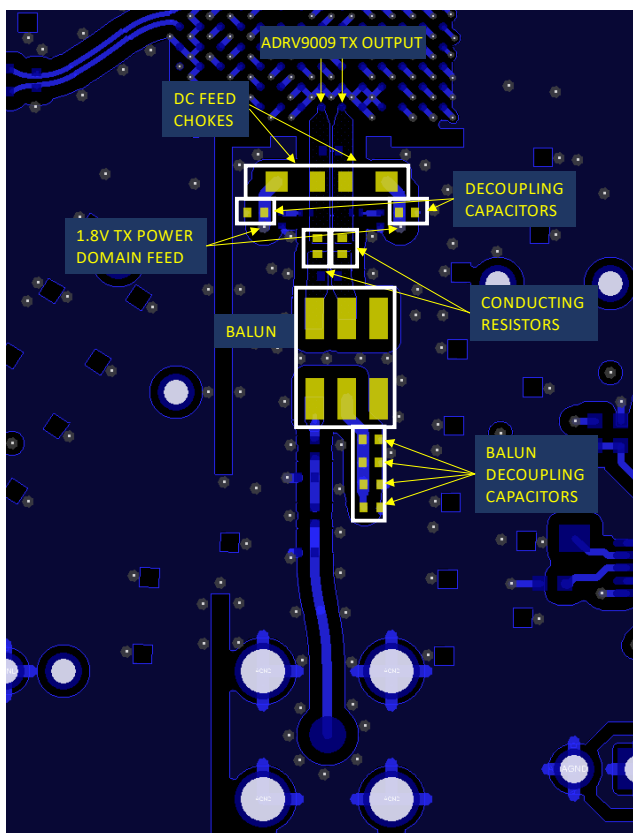
Figure 443. Transmitter DC Chokes and Balun Feed Supply
