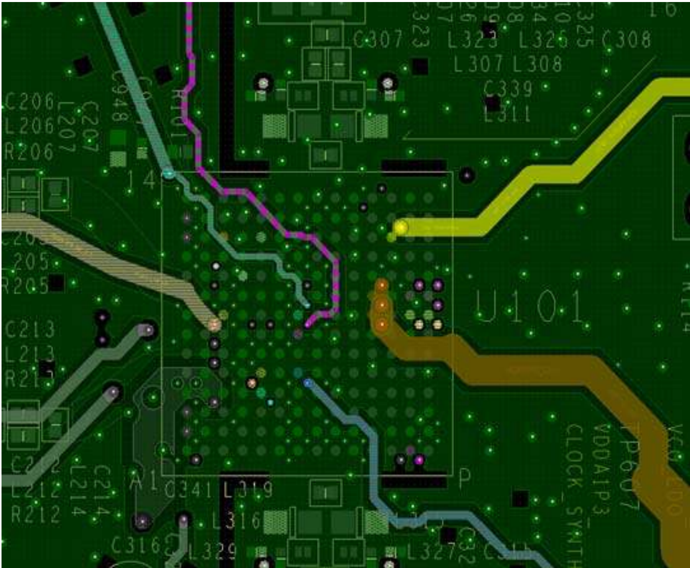
Figure 436. Layout Example of Power Supply Domains Routed with Ground Shielding (Layer 12 to Power)
