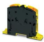
High-current terminal block, nom. voltage: 1000 V, nominal current: 232 A, connection method: Power-Turn connection, 1 level, cross section: 25 mm<sup>2</sup> - 95 mm<sup>2</sup>, mounting type: direct screw connection, color: black/yellow
