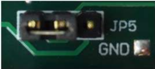
Figure 2A. (JP5: Pin 1 - 2 to Voltage Regulators)
