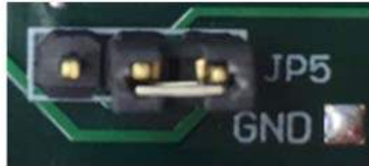
Figure 2B. (JP5: Pin 2 - 3 to Banana Jack)
