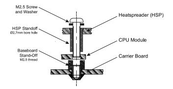
Top mounting scenario uses the bore hole version heatspreader and requires threaded standoffs on the carrier board.
