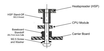
Bottom mounting scenario uses the threaded version heatspreader and requires bore hole standoffs on the carrier board.
