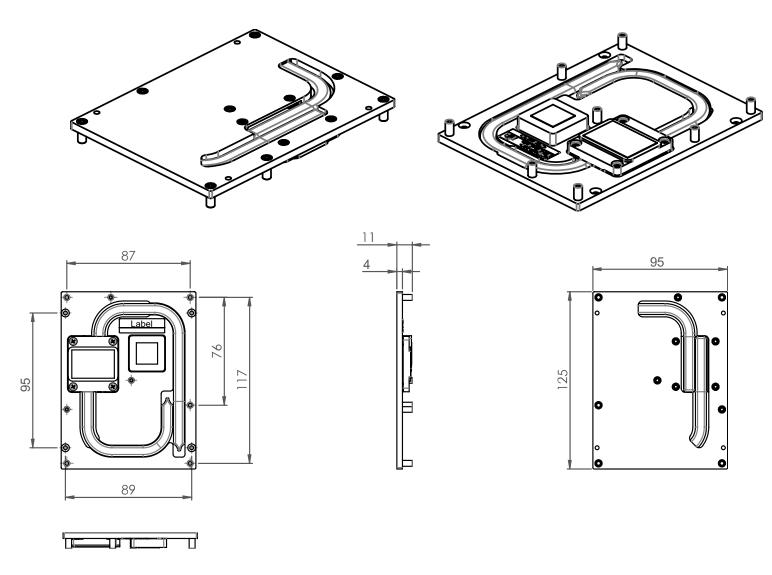
Mounting standoffs and holes are placed symmetrically [mm]
