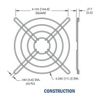
Rings: .063 (1.60) wire diameter CAT. NO. 8448 Ribs: .063 (1.60) wire diameter
