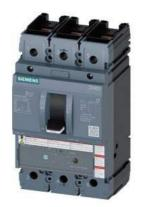
circuit breaker 3VA5 UL frame 250 breaking capacity class C 100kA @ 480 V 3-pole, line protection TM240, ATAM, In=200A overload protection Ir=160A ...200A short-circuit protection Ii=5...10 x In nut keeper kit on both sides
