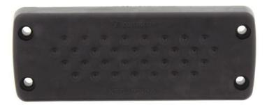
Cable entry with membrane for unassembled cables, Mounting type: Screw, Length: 147 mm, Width: 58 mm, IP66, Colour: Black
