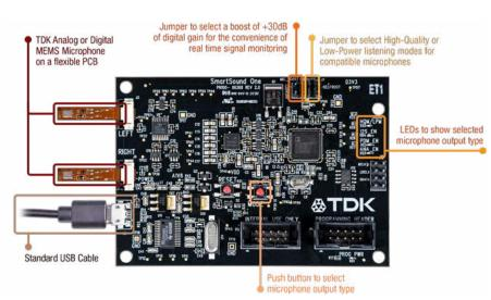
SmartSound One features an EEPROM to load the factory default DSP program on power up, making it a plug-and-play solution. There are two parallel signal processing paths for analog and digital microphones which the user can select using the 'mode' button which is routed through the DSP and the on-board USB audio codec to send audio data packets over USB.
