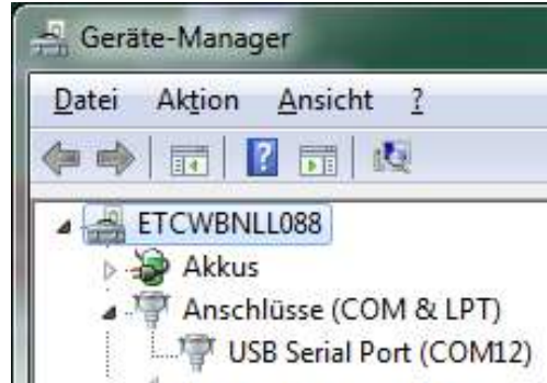
Figure 9: The Demo Kit must be visible as a virtual ComPort in the Windows device manager.
