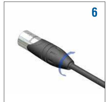
Thread the nut (Backshell) onto the shell (Torque 0.8Nm - 1.2Nm) to activate the cable clamp and close the connector assembly.
