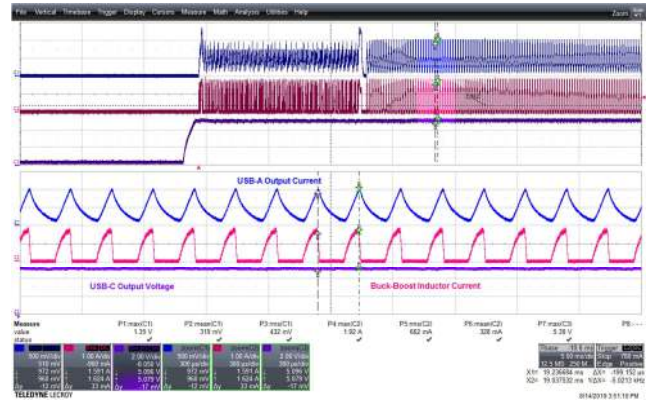
Figure 124 – 265 VAC 60 Hz, USB-A Start-up Short. CH1(Blue): I_{USB-Ar} 0.5 A / div., 5 ms / div. CH2(Pink): I_{L3r} 1 A / div. CH3(Violet): V_{USB-C} 2 V / div.
