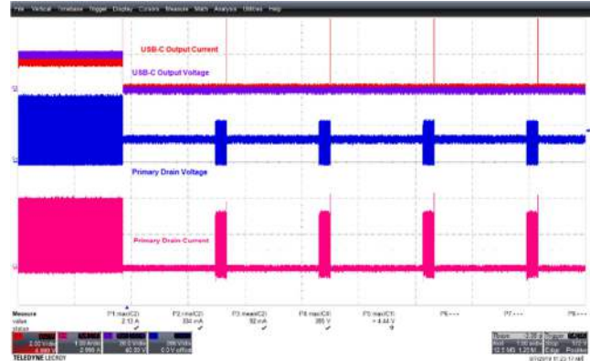
Figure 120 – 265 VAC 50 Hz, USB-C Full Load Short. CH1(Red): I_{\text{USB-C}} , 2 A / div., 1 s / div. CH2(Pink): I_{\text{DRAIN}} , 1 A / div. CH3(Violet): V_{\text{USB-C}} , 20 V / div. CH4(Blue): V_{\text{DRAIN}} , 200 V / div.
