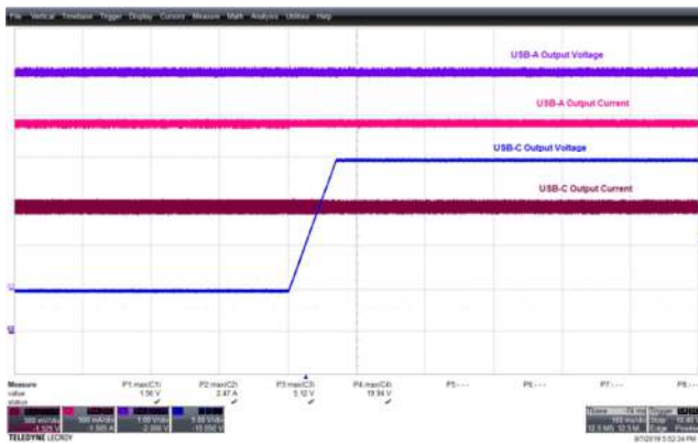
Figure 89 – 90 VAC 60 Hz, 5 – 20 V USB-C Step CH1(Brown): I_{USB-C} , 500 mA / div. CH2(Pink): I_{USB-A} , 500 mA / div. CH3(Violet): V_{USB-A} , 1 V / div., 500 ms. CH4(Blue): V_{USB-C} , 5 V / div. Remark: No overshoot/undershoot.
