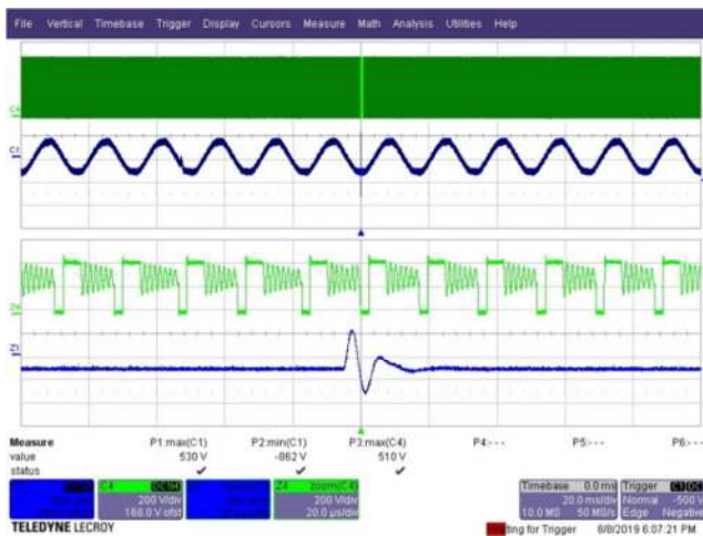
Figure 164 – 230 VAC 50 Hz, 2.5kV Ring Wave L/N. Injection Phase: 90°. Upper: V DRAIN , 200 V / div. Lower: V IN , 500 V / div., 20 ms / div. VDS = 510 V.
