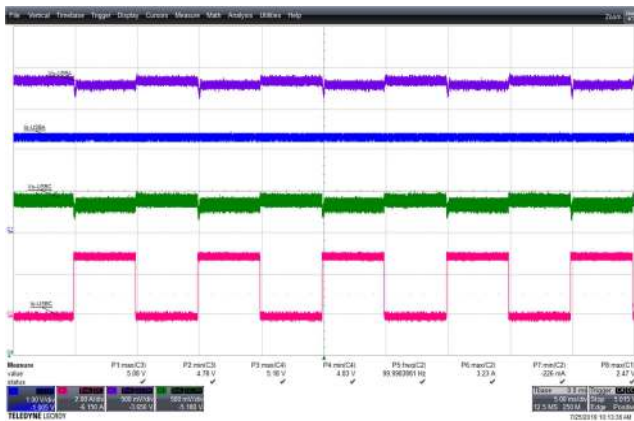
Figure 93 – 90 VAC 60 Hz, 0-3 A USB-C Transient Load CH1(Blue): I_{USB-A} , 1 A / div., 5 ms / div. CH2(Pink): I_{USB-C} , 2 A / div. CH3(Violet): V_{USB-A} , 0.5 V / div. CH4(Green): V_{USB-C} , 0.5 V / div.
