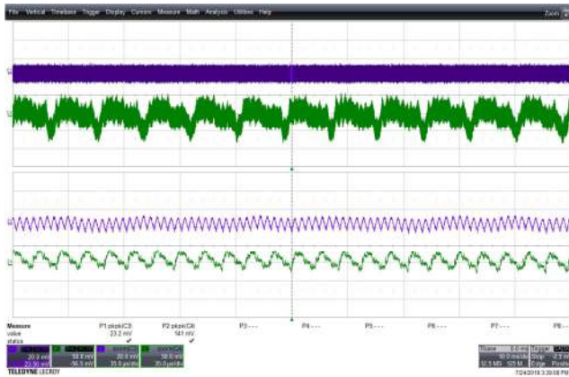
Figure 115 – 90 VAC 60 Hz, Full Load Normal. Upper: V_{USB-A} , 50 mV / div., 10 ms / div. Lower: V_{USB-C} , 50 mV / div. V_{RIPPLE(USB-A)} = 23.2\text{ mVpp} . V_{RIPPLE(USB-C)} = 141\text{ mVpp} .
