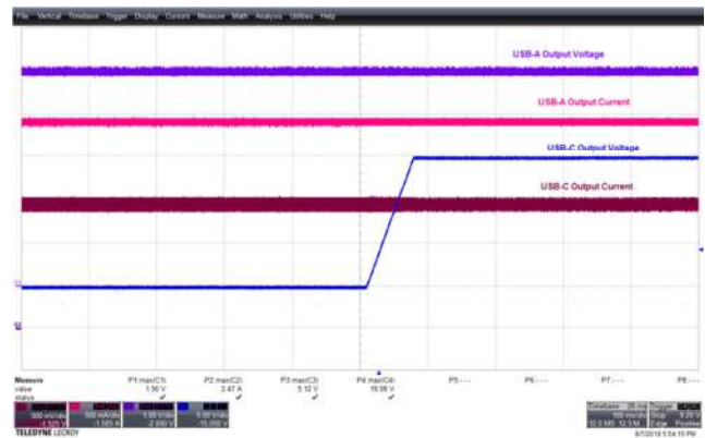
Figure 90 – 265 VAC 60 Hz, 5 – 20 V USB-C Step CH1(Brown): I_{USB-C} , 500 mA / div. CH2(Pink): I_{USB-A} , 500 mA / div. CH3(Violet): V_{USB-A} , 1 V / div., 500 ms. CH4(Blue): V_{USB-C} , 5 V / div. Remark: No overshoot /undershoot.
