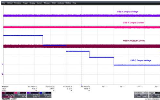
Figure 87 – 90 VAC 60 Hz, 20 V - 15 V - 12 V - 9 V - 5 V. CH1(Brown): I_{USB-C} , 500 mA / div. CH2(Pink): I_{USB-A} , 500 mA / div. CH3(Violet): V_{USB-A} , 1 V / div., 500 ms. CH4(Blue): V_{USB-C} , 5 V / div. Remark: No overshoot/undershoot.
