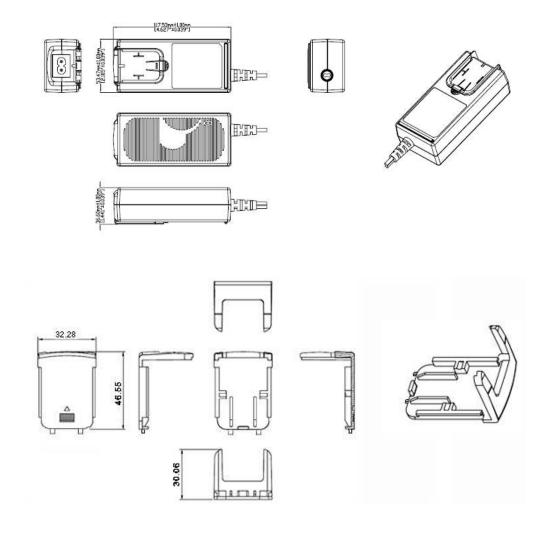
Unit shipped without an installed input plug.
