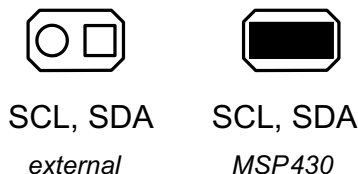
Figure 4. I 2 C Interface Jumper Settings
