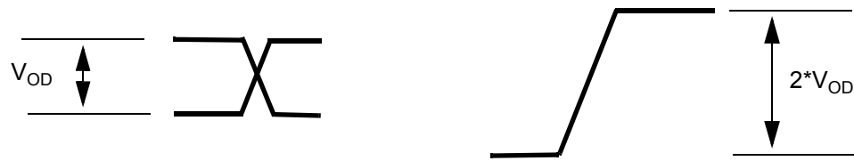
Figure 19 - Differential Output Voltage Parameter
