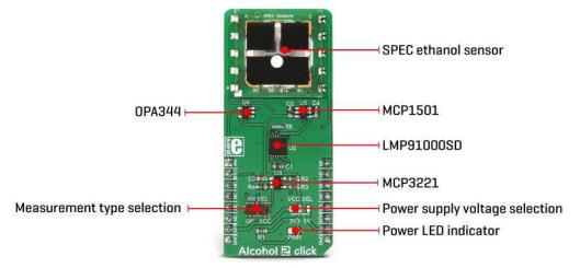
Although very reliable and accurate, this sensor is great for building relative gas sensing applications. For example, it can detect increased levels of ethanol gas. However, when developing applications for the absolute gas concentration, the sensor needs to be calibrated and the measurement data needs to be compensated.
