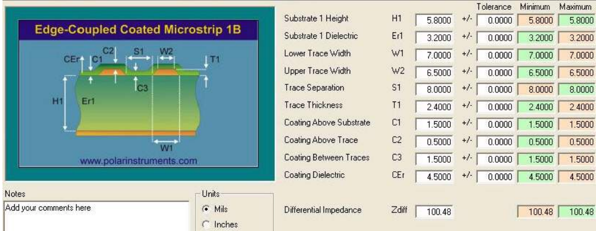
Figure 8. DS50PCI401EVK 100 Ohm Differential Microstrip
