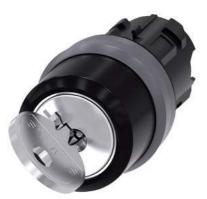
RONIS key-operated switch, 22 mm, round, plastic with metal front ring, lock number SB30, with 2 keys, 2 switch positions O-I, latching, actuating angle 90°, 10:30h/13:30h, key removal I, possible special locks: SB31, 421, 455, with laser labeling, upper case and lower case, always upper case at the beginning of the word
