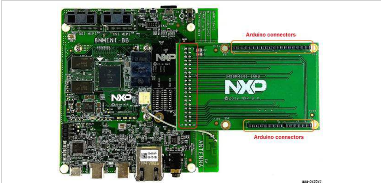
Figure 2. The IMX8MMINI-IARD interposer board attached to the EVK
