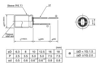
%1 In case  $\phi$ 10 × 40, lead dia  $\phi$ d=0.8 %2 In case L>25 for the  $\phi$ 12.5 dia unit, lead dia  $\phi$ d=0.8
