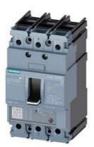
circuit breaker 3VA5 UL frame 125 3-pole, starter protection TM120M, AM, In=7A without overload protection short-circuit protection li=3...7 x In cable connection on both sides
