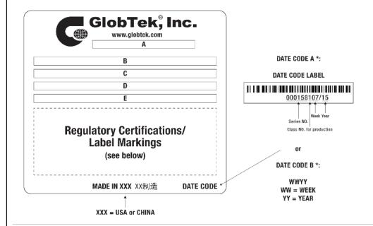
A=ICT/ITE Power Supply B=P/N: (料号) WR9MA1200MICB-F(R6W) C=Model (型号) GT-86060-0605-W2E D=Input (输入)100-240V~, 50/60Hz, 0.2A E=Output (输出)5.0 V == 1.2 A, 6.00W
