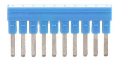
Insulated cross-connector, No. of poles: 10, Mounting type: Plug in, Width: 40.9 mm, Colour: Blue
