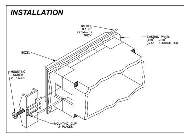
The Apollo Process Voltmeter is designed to be panel-mounted with a gasket to provide a water-tight seal. Two mounting clips and screws are provided for easy installation. Consideration should be given to the thickness of the panel. A panel which is too thin may distort and not provide a water-tight seal. (Recommended minimum panel thickness is 1/8".)
