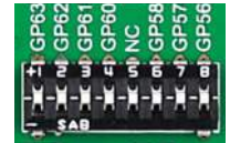
Figure 6-3: Tri-state DIP switch on PORT00-07
