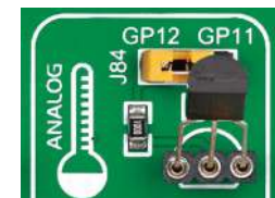
Figure 24-4: LM35 correctly placed in socket
