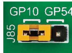
Figure 19-1: Jumper J85 reroutes the AN pin on the second mikroBUS™ socket from GP10 to GP54
