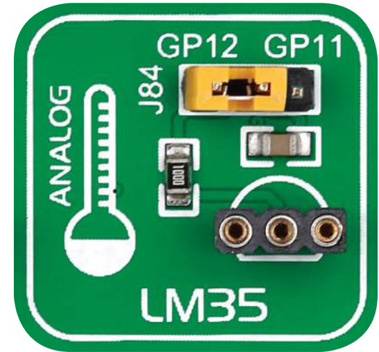
Figure 24-2: Choose between two analog input lines to use with LM35, with jumper J84
