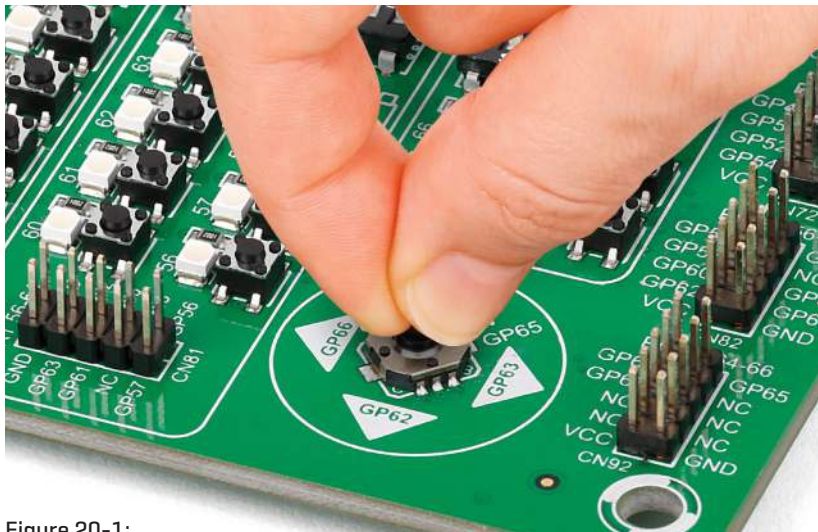
Figure 20-1: Navigation switch is an intuitive solution for browsing through on-screen menus.
