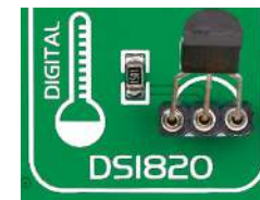
Figure 23-3: DS1820 correctly placed in socket
