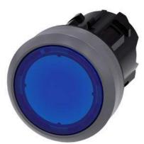
Illuminated pushbutton, 22 mm, round, plastic with metal front ring, blue, pushbutton, flat, latching, Push-to-release mechanism, with laser labeling, symbol number according to, ISO 7000 or IEC 60417
