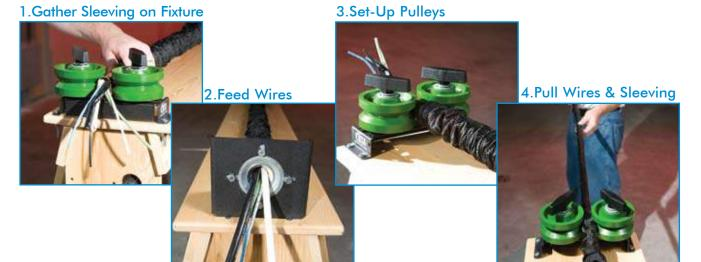
This completely modular system allows production level installation of braided sleeving over wire and cable bundles of virtually unlimited length. The system is simple to set up and interchangeable components accommodate diameters up to 2". For more information about this product contact your Account Representative.
