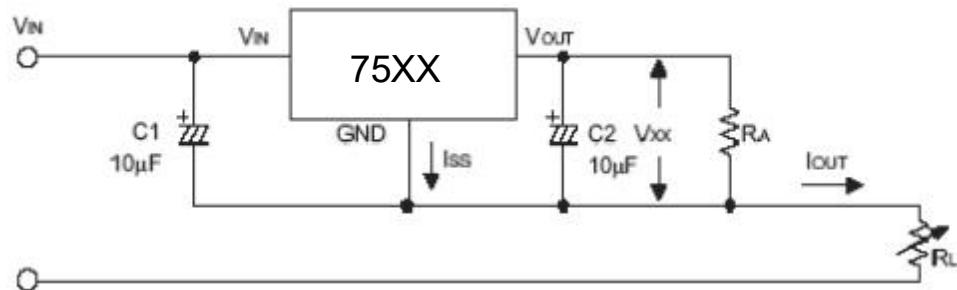
$$I_{OUT} = V_{XX}/R_X + I_{SS}$$
