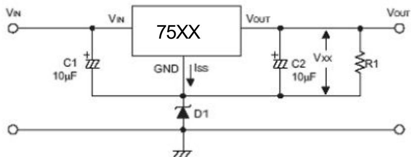
$$V_{OUT} = V_{XX} + V_{D1}$$
