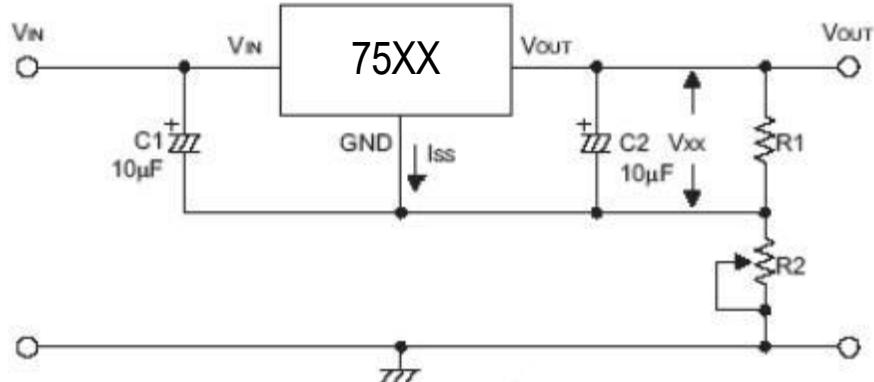
$$V_{OUT} = V_{XX} \left(1 + \frac{R_2}{R_1}\right) + I_{SS} \cdot R_2$$
