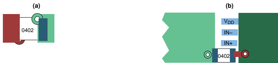
Figure 18. Typical Decoupling Capacitor Layouts
