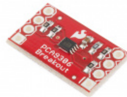
SparkFun Level Translator Breakout - PCA9306
