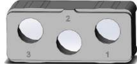
Insert Name 3T3 (1) Insert Code Z 3 x size 8 BMA pin contacts
