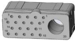
Insert Name 20C1 Insert Code M 19 x size 20 contacts 1 x size 5 coax contact
