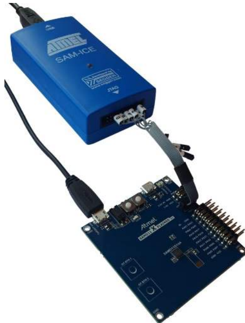
Figure 5-6. SAM-ICE using a Squid Cable
