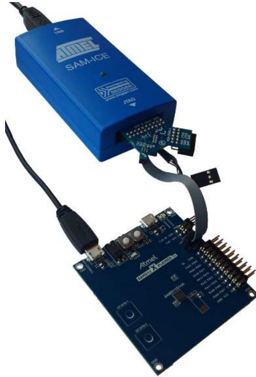
Figure 5-7. SAM-ICE using an Atmel-ICE Adapter
