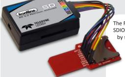
The Frontline SD Protocol Analyzer includes powerful Frontline software and the SD/SDIO/SPI/ MMC hardware interface.
