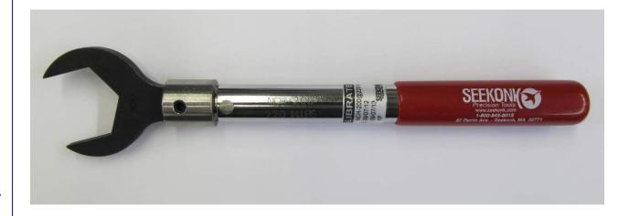
Pre-set at factory to desired value within a  $\pm$ /- 4% tolerance. When preset torque value is achieved, a distinct click is felt and heard, followed by a sudden release into several degrees of free movement. Ideal for applications in which one torque value is used extensively. Compact design makes these tools invaluable in hard to reach locations. Tools automatically reset when torquing- force is removed.
