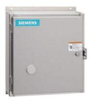
Non-reversing NEMA contactor, Size 2, Three phase full voltage, Contactor amp rating 45A, 3 wire (NO aux included), 190-220/220-240V 50/60Hz coil, Non-combination type, Encl NEMA type 4X 304 S-Steel, Water/dust tight noncorrosive, Extra-wide enclosure
