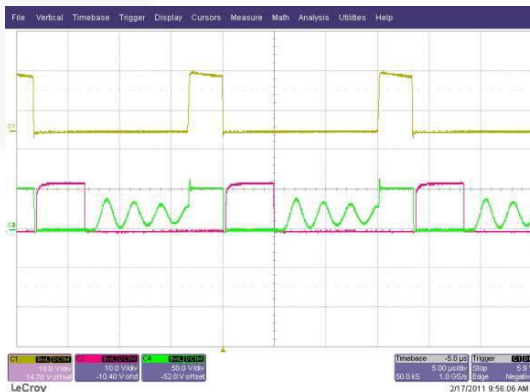
Figure 6. FAN6754AMR+FAN6204MY 115V/60Hz, 20% Load (Ch1: Gate, Ch2: Gate_SR, Ch4: V dS )
