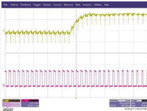
Figure 4. FAN6754AMR+FAN6204MY 115V/60Hz, Overshoot (Ch1: V OUT , Ch2: Gate)
