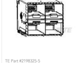
TE Part #2198325-5 zSFP+ STACKED 2X2 RECEPTACLE ASSEMBLY
