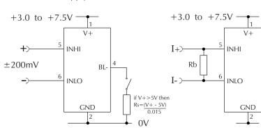
Measuring an input voltage referenced to a floating supply, i.e. the input voltage and the meter's power supply are isolated from each other. Ensure solder link LCOM is closed. Measuring a current from a circuit which is floating with respect to the DPM's supply, i.e. the current and the meter's power supply are isolated from each other. Ensure solder link LCOM is closed.
