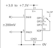
Measuring a single ended input voltage referenced to supply, i.e. the input voltage and the meter's power supply share the same 0V rail. Ensure solder link LCOM is open.
