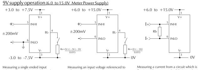
Measuring a single ended input voltage referenced to supply, i.e. the input voltage and the meter's power supply share the same 0V rail. Ensure solder link LCOM is open. Measuring an input voltage referenced to a floating supply, i.e. the input voltage and the meter's power supply are isolated from each other. Ensure solder link LCOM is closed.
