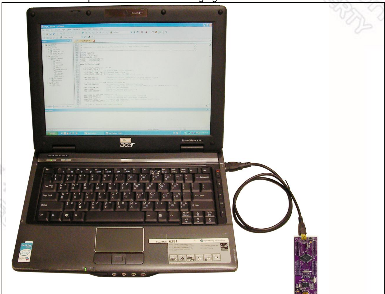
Figure 4-1 NuTiny- SDK-NUC220 Hardware Setup
