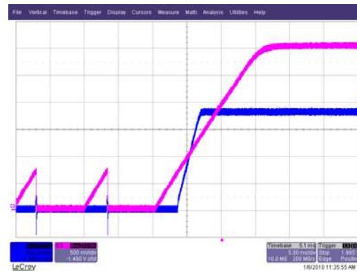
Fig. 12. Short (Hiccup) Recovery Ch 2 :V o , Ch 3 :V SS
