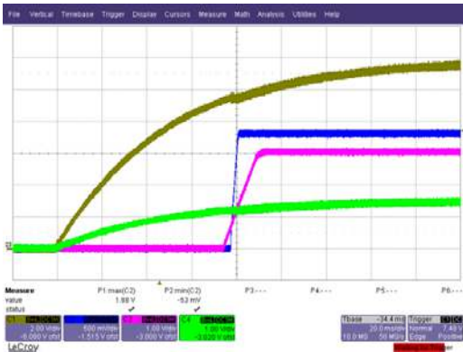
Fig. 7. Start up at 6A Load Ch 1 :V in , Ch 2 :V o , Ch 3 :V ss , Ch 4 :Enable
