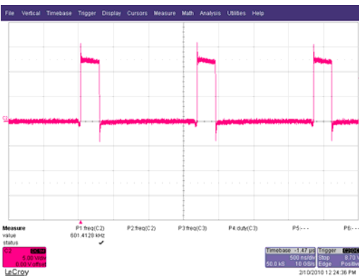
Fig. 11. Inductor node at 6A load Ch 1 :LX
