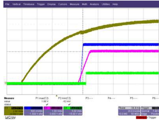
Fig. 8. Start up at 6A Load, Ch 1 :V in , Ch 2 :V o , Ch 3 :V ss , Ch 4 :V PGood
