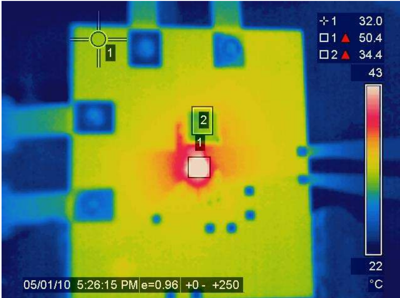
Fig. 17: Thermal Image at 6A load Test points 1 and 2 are IR3842A and inductor, respectively.
