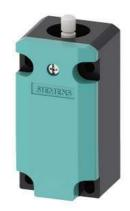
Position switch Basic switch plastic 40 mm according to EN 50041 Increased corrosion protection Device connection 1 x (M20 x 1.5) 1 NO/2 NC slow-action contacts functional at -40  $^{\circ}$ C Shock and vibration test according to EN 61373, Category 1B
