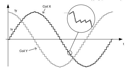
Figure 18. Current Waveforms in Motor Coils X and Y in 1/16<sup>th</sup> Micro-Step Mode
