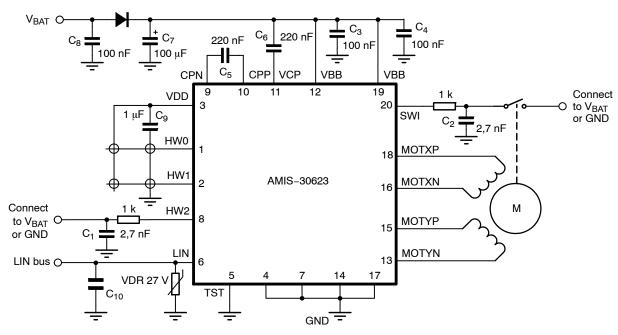
Figure 6. Typical Application Diagram for SO Device
