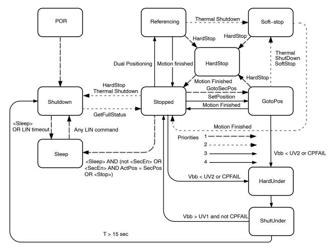
Figure 16. Simplified State Diagram
