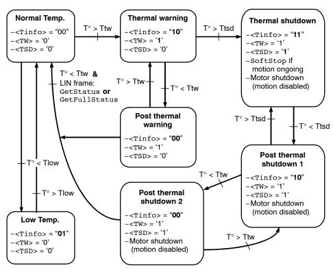
Figure 14. State Diagram Temperature Management
