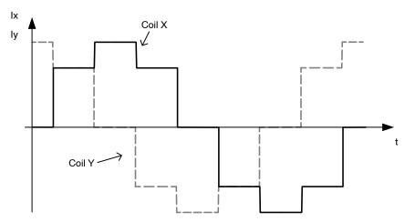
Figure 17. Current Waveforms in Motor Coils X and Y in Halfstep Mode
