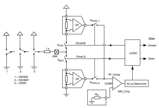
Figure 12. Simplified Schematic Diagram of the SWI Comparator
