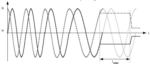
Figure 19. Motor Stopping Phase
