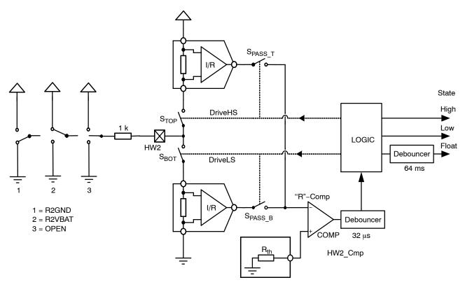
Figure 10. Simplified Schematic Diagram of the HW2 Comparator
