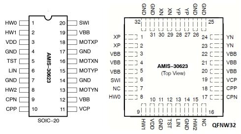
Figure 2. SOIC-20 and QFNW32 Pin-out
