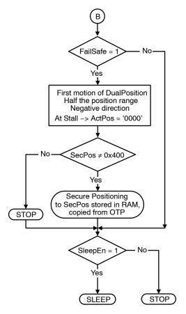
Figure 25. Case B: LIN Lost at or During Start-Up
