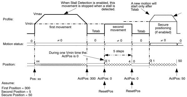
Figure 8. Dual Positioning
