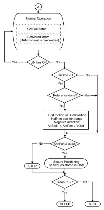
Figure 24. Case A: LIN Lost During Normal Operation
