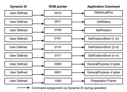
Figure 22. Principle of Dynamic Command Assignment
