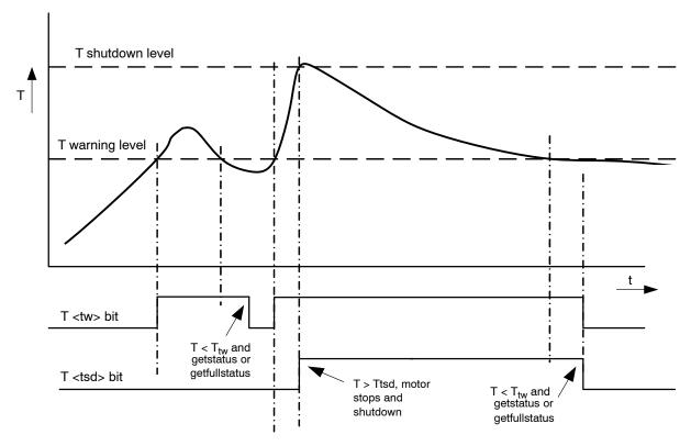
Figure 15. Illustration of Thermal Management Situation
