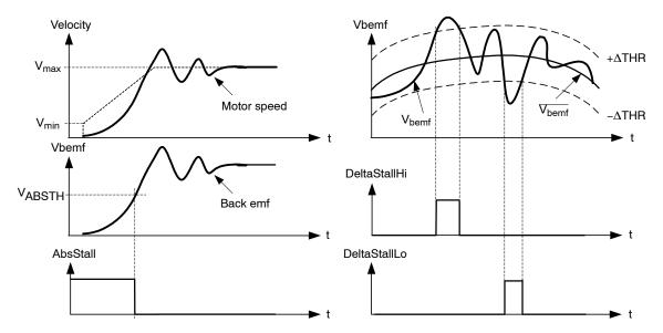
Figure 20. Triggering of the Stall Flags in Function of Measured Backemf and the Set Threshold Levels
