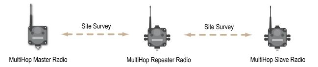
After MultiHop radios are communicating to their parents, the network formation information is transmitted back to the radio master, creating a path that is stored in each parent radio's routing tables. Each parent radio stores only one link or step along a path to an end radio. The routing information for non-MultiHop Modbus slave devices is stored as the devices are accessed by the host system.
