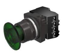
30mm BlackMax, Epoxy Coated Corrosion Resistant Complete Metal Unit Illuminated Twist-to-Release Full Voltage, 6V AC LED Lamp Mushroom Head Cap Small 1.79" (45 mm) Plastic Cap, Green 2 Position Maintained, Twist-to-Release with 1 N.O. - 1 N.C. Heavy Duty Contacts, A600/P600 UL Listed, CSA Certified NEMA 1,3,3R,4,4X,12,13 & Automotive Standards
