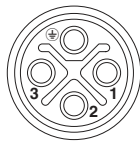
Connector pin assignment of M12 socket, 4-pos., S-coded, view of socket side
